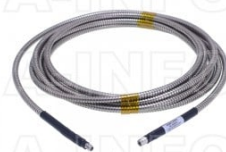
2.4M-2.4F-B020S-5000 Flexible Cable Assembly 5000mm DC-50GHz 2.4mm Male to 2.4mm Female
